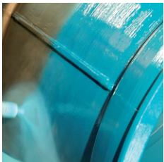
Applying powder using a spray gun
