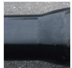
Appearance of the TT-PE coating for DN ≤ 500
