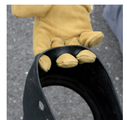
These holes make the sleeve easier to fit. Handy!
